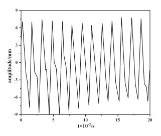
**FIGURE 5** Time domain waveform of spindle vibration of NC machine tool when copper bar contacts
