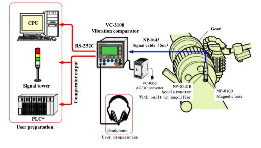
FIGURE 1 Schematic diagram of mechanical manufacturing vibration system detection
