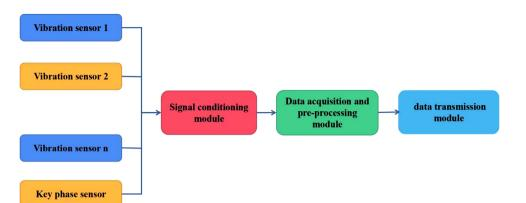
FIGURE 3 Hardware structure block diagram of spindle vibration monitoring system of NC machine tool
