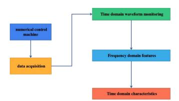
FIGURE 2 Structural block diagram of spindle vibration monitoring system of mechanical NC machine tool
