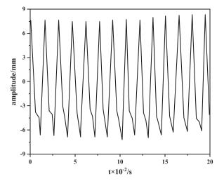
**FIGURE 4** Time domain waveform of spindle vibration of NC machine tool without copper bar contact
