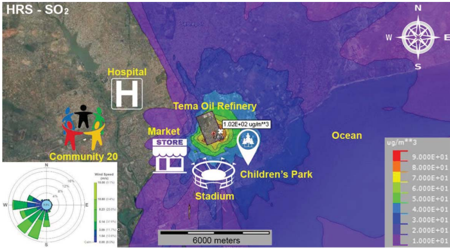
Figure 4. Distribution patterns of maximum hourly SO 2 emissions during HRS in TOR area.
