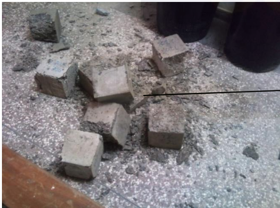
Figure 3.6 Crushed concrete cubes.
