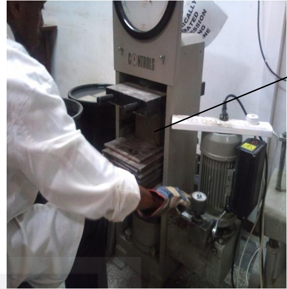
Figure 3.4: Compression testing machine Figure 3.5: A concrete cube undergoing test
