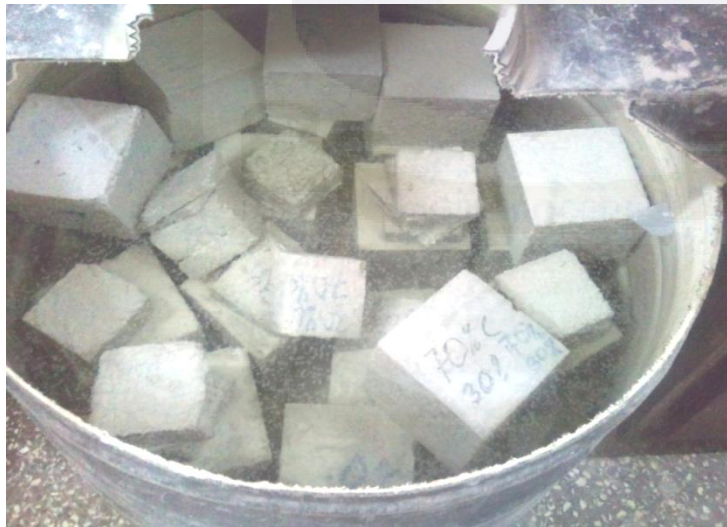
Figure 3.2: Water bath containing labeled concrete cubes and slabs.
