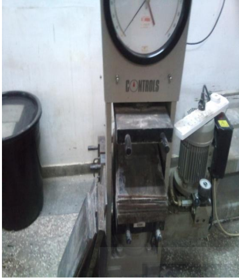
Figure 3.4: Compression testing machine Figure 3.5: A concrete cube undergoing test
