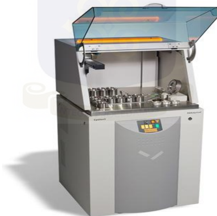
Figure 3.3: Epsilon 5 XRF machine showing sample chamber
