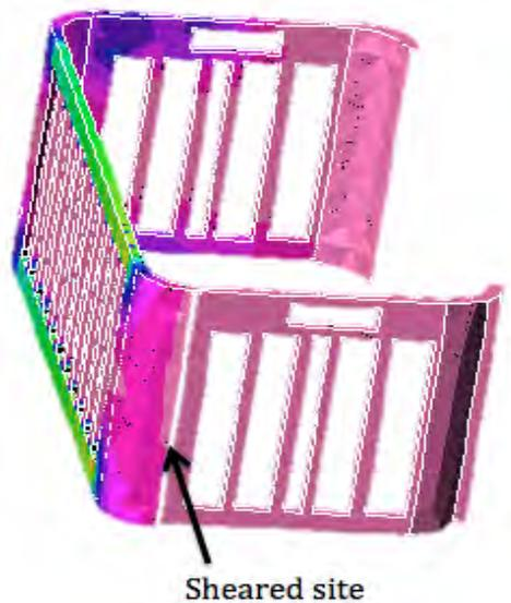
Fig. 6. Fracture due to a 4 kN force
