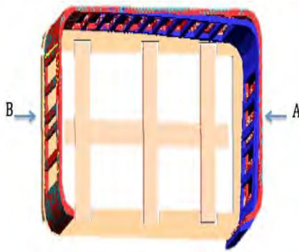
Fig. 5. Result of mechanical test on a virtual model. The direction of force applied is indicated by the arrows. The blue colour shows distortion relative to the true shape of the crib under the action of a 2 kN force
